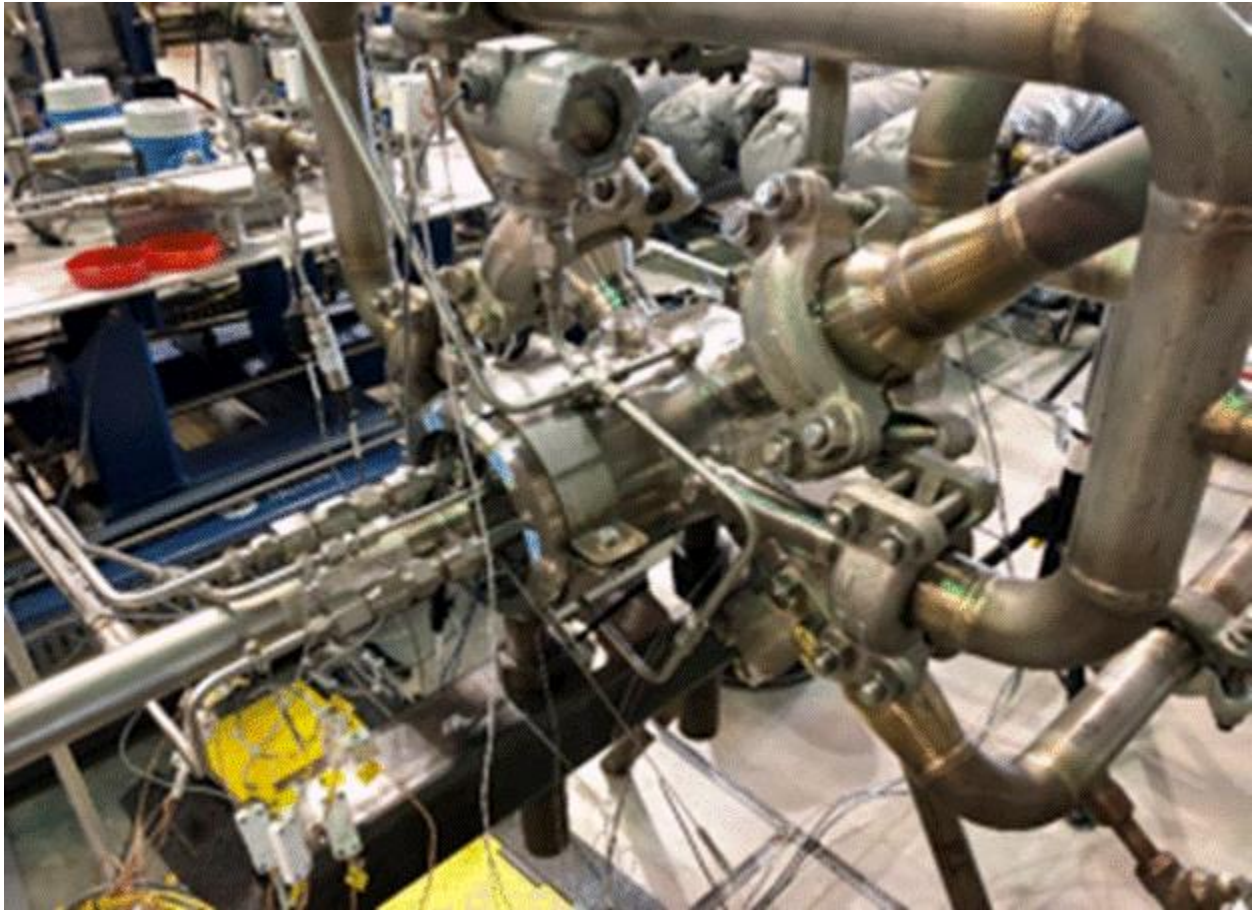
Figure 3 – PTT's Turbo-Pump Under Test at SNL
